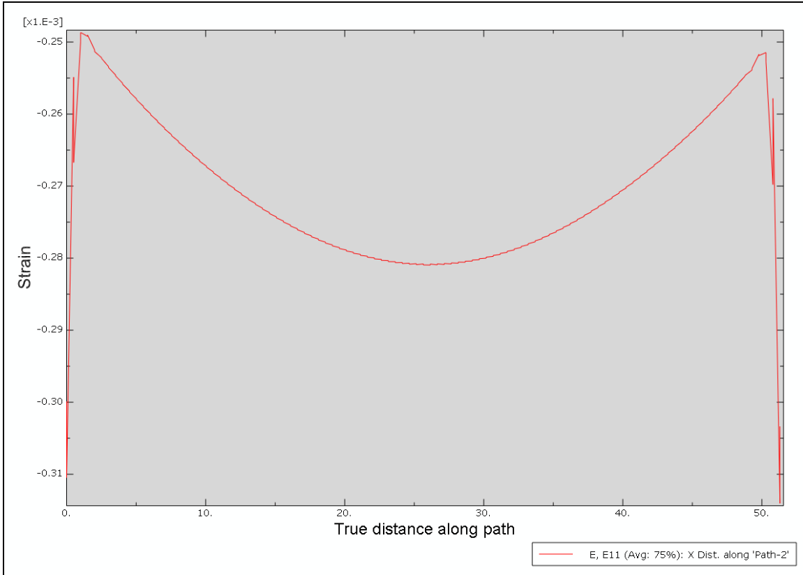
Figure 71: Strain along length of coating at coating beam interface in the center of the beam
